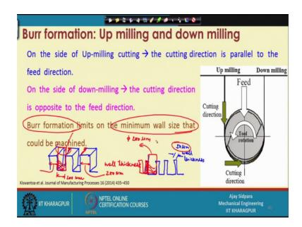
So, that is why it is called up milling. And if you consider the second one in the side of the down milling in this particular direction the cutting direction is opposite to the feed directions.
