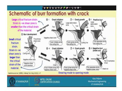
That may ductile material and brittle material forms burr in different, different ways. And in this case, we have seen that, these are the positive burrs because it removes material of
