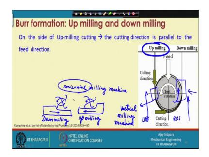
So now coming to 2 different theories; that is, one is the up milling and another is the down milling. So, these 2 things are different in this sense that how the cutter is approaching the work piece material. So, let us see that thing. So, this is the case of a slot cutting in the micro milling operation. So, we know that there are 2 ways.
