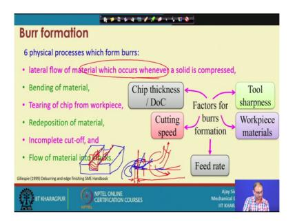
Then what are the ways because of that burrs are farming into the workpiece. So, let us see those things. So, factors of the burr formation. So, one is the tools sharpness play important role because if you are machining with a blunt tool at that time we know that, you are cutting edge radius is very less compared to the uncut chip thickness.
