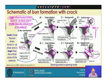
So now, earlier slide was the before the crack propagation and now this one is the with crack propagation. So, let us take this particular image again to the next slide and so can we can understand what things are shown. This is the earlier figures whatever it has created here, correct. So, this is the same figure. So, now, or objective is to cut material from these, but and these also. So, this is the extra thing.
