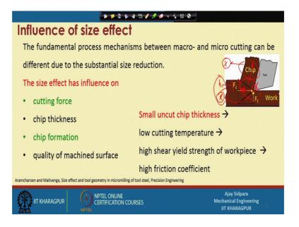
So, now how the what is the effect of size effect influence of size effect on the different type size effect means when you scale down the tool when you scale down the uncut chip
