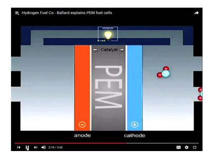
If the catalyst splits the hydrogen molecule into protons and electrons, if the protons can pass through the membrane the electrons cannot and have to pass through an external circuit creating useful electricity. On the oxygen side of the membrane the protons and the electrons react with oxygen from the air in the presence of a second catalyst layer generating water and heat.
