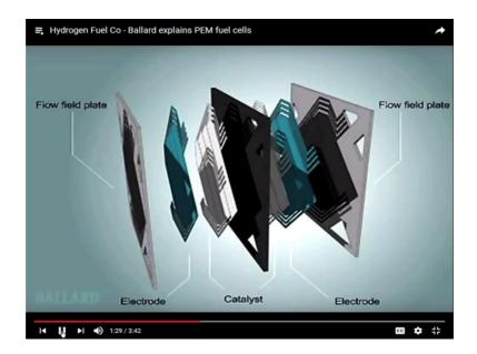
A single PEM fuel cell is made up of 2 plates, 2 electrodes and 2 thin layers of platinum based catalyst separated by a plastic membrane which when fed with the fuel reacts electrochemically to create electricity.
