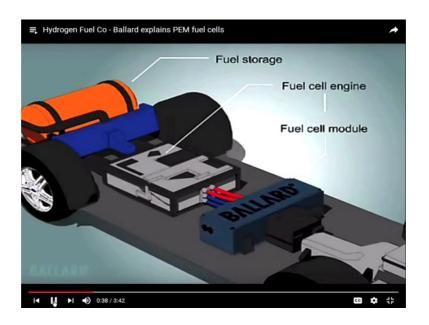
A fuel cell engine consists of the proton exchange membrane or PEM fuel cell module coupled with the systems required in a typical automotive engine.
