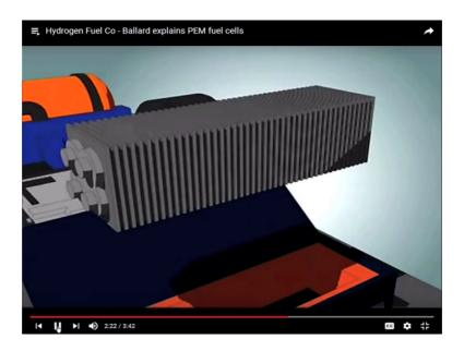
By stacking, together single cells like slices in a loaf of bread. You make a fuel cell stack to produce the required amount of power just like your car fuel cells need fuel to operate.
