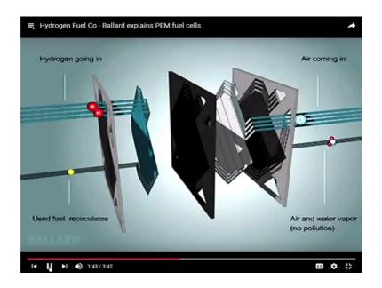
Hydrogen from an onboard storage tank and oxygen from air are fed through channels in the plates hydrogen flows on one side of the membrane air on the other.
