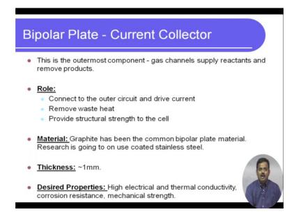
And the bipolar plate is the current collector that role is to connect outer circuits and drive the current it removes a waste heat and it provides structural strength to the cell so this is a thickest part which is 1 millimeter and as I said on both sides of the bipolar plate because we are sandwiching many of these cells one after the other. The bio polar plates are such that there are channels on both sides in that figure that I showed a few slides back it showed channels only on one side.
