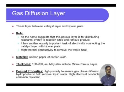
Gas diffusion layer as the name suggests, this is a porous layer and it is required for distributing the reactants evenly at the reaction sites and later remove the products also after the reactions happen at the catalysts. But however, it is also another equally important task of electrically connecting the catalyst layer with the bipolar plate clear, because this is what is actually sandwiched between the bipolar plate and the catalysts.
