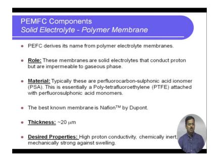
So, let us move on let us move on to some of the components that we saw in a PEM fuel cell. So what is the first one most important is the solid electrolyte which is a polymer membrane so polymer electrolyte membrane that is where the PEFC or PEMFC derives it is name from I again want to clarify something PEFC and PEMFC are used interchangeably proton exchange fuel cell is actually proton exchange membrane fuel cell.
