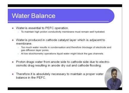
I would just end this by talking a little bit about water balance look water is essential for PEFC operation, the proton membrane has to be proton elect electrolyte membrane proton exchange membrane has to be well hydrated for the movement of the protons, but also the water is produced in the cathode catalyst which is adjacent to the membrane. But if there is too much of water what will happen is there will be blockage of the electrode and gas diffusion layer pores.
