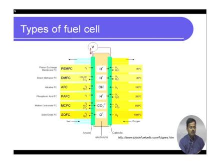
So, if we talk about fuel cells as we said, a typical fuel cell will have two electrodes and an electrolyte same as battery. So the fuel cell depending on what is there can be of several types which is shown pretty nicely in this schematic diagram. So, we have proton exchange membrane fuel cell which is PEMFC, PEM or PEM fuel cell is sometimes it is called and we are going to discuss this in details.
