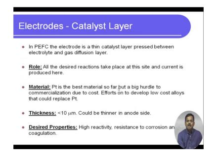
The second one are the electrodes which is the catalyst layer. So those are the electrodes the catalysts are the electrodes. So the electrode is a thin catalyst layer that is pressed between the electrolyte and the gas diffusion layer let us just go back to few slides this is the electrode that we are talking about press between the electrolyte and the GDL or the gas diffusion layer.
