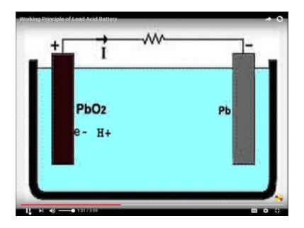
The hydrogen ions when reach at lead peroxide plate they receive electrons from it and become hydrogen atom which again attacked lead peroxide.
