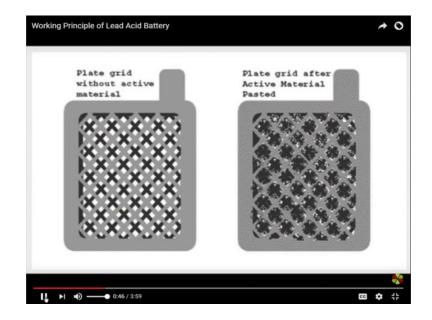
The negative Plate of lead acid battery is made of pure lead in soft sponge condition, dilute sulphuric acid used for lead acid battery as ratio of water is to acid equal to 3 is to 1.
