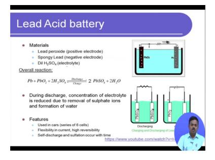
So what is the lead acid battery? It has 2 electrodes, one is Lead it is actually not solid leads what we call spongy lead which is a negative electrode. And lead peroxide which is a positive electrode the electrolyte is dilute sulfuric acid.
