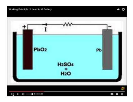
A load is connected externally between these plates in diluted sulfuric acid.
