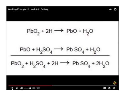
And formed lead oxide and water this lead oxide reacts with sulfuric acid and forms lead sulfate and water.
