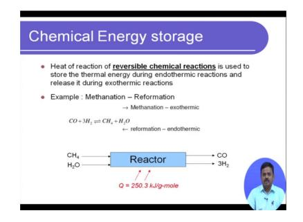
Next what we are going to look at is chemical energy storage. So, previous one was electrochemical you had a certain electrolyte and an anode and cathode immersed in it and we were using electrical energy also. Because there was movement of ions etcetera this is completely chemical energy storage and in some way you can even argue that this is thermal energy storage because the form in which the energy is stored or released is again heat.
