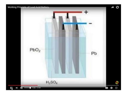
The lead acid storage battery is formed by dipping lead peroxide plate and sponge lead plate in dilute sulfuric acid.
