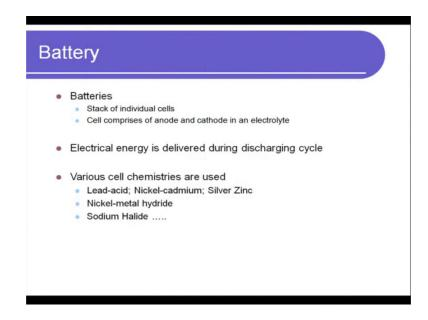
So batteries as we know it are a stack of individual cells. When we talk about battery we go to a shop and say let us buy a battery we typically buy one cell. Some applications just one cell is good enough, but in most applications it is not. I mean even in your TV remotes most of the times we need two such batteries, many other appliances in a torch probably we need three of them if it is a powerful one.
