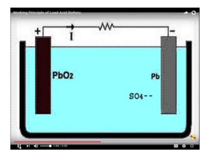
Negative sulfate ions are moving freely in the solution so some of them will reach to pure lead plate where they give their extra electrons and become radical sulfate.
