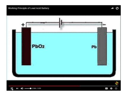
Now, we will disconnect the load and connect lead sulfate covered lead peroxide plate with positive terminal of an external dc source and lead peroxide covered lead plate with negative terminal of that dc source.
