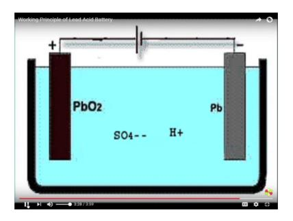
Negative sulfate ions move towards the electrode connected with the positive terminal of dc source, where they will give up their extra electrons and become radical sulfate.
