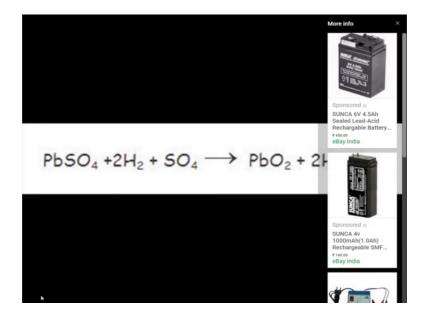
This radical sulfate reacts with lead sulfate of anode and forms lead peroxide and sulfuric acid, hence by charging the lead acid storage battery cell becomes ready for discharging alright.
