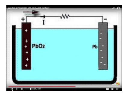
There would be an inequality of electrons between these 2 plates. Hence there would be a flow of current through the external load between these plates for balancing this inequality of electrons this process is called discharging of lead acid battery.
