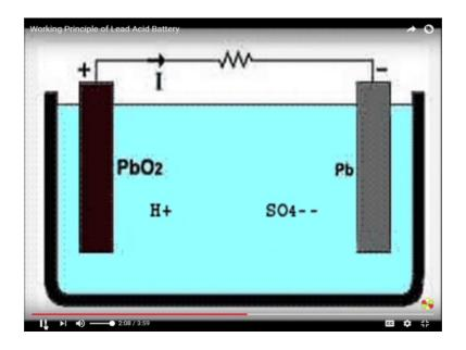
As positive hydrogen ions take electrons from lead peroxide plate and negative sulfate ions give electrons to lead plate.
