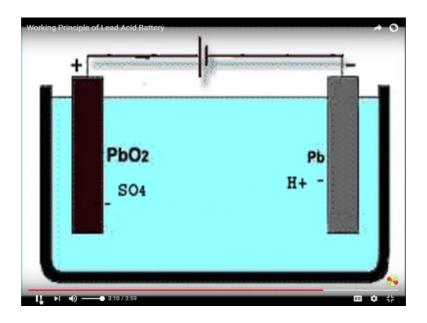
Here each hydrogen ion takes 1 electron from that and becomes hydrogen atom.
