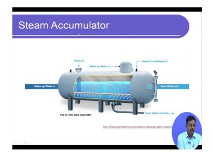
So, as it is extracted out it is fed into what is called a Steam Accumulator? A Steam Accumulator as you can see is actually a cylindrical vessel, it can be quite large with and where the steam is injected through these injecting nozzles that go through it. It is actually the steam accumulator is a big vessel that consists of water typically at a high temperature and in that the steam is injected through these nozzles.
