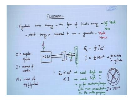
As we know that I would write down something that some of the points that we discussed flywheel stores energy in the form of kinetic energy and this definitely is going to be during off peak hours, right and the stored energy is released to run a generator and this is during peak hours, clear. So, this is what we saw.
