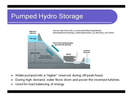
So, the first thing that we are going to talk about is pumped hydro electric storage or pumped hydro. So, what is pumped hydro? So, pumped hydro storage actually means
