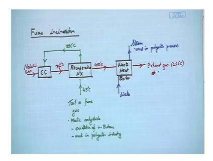
I will say what we are doing here incinerator. So, let me draw an example where have a combustion chamber then a recuperative heat exchanger which I believe you all know very well now that you have studied heat exchanger as part of this course then we have what we called a waste heat boiler.
