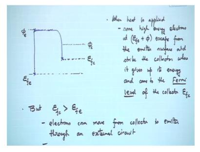
So, let me say that this is one level, this is the energy level, and I am calling it the Fermi level of the emitter. Similarly this is one level and I am going to call it the work function
