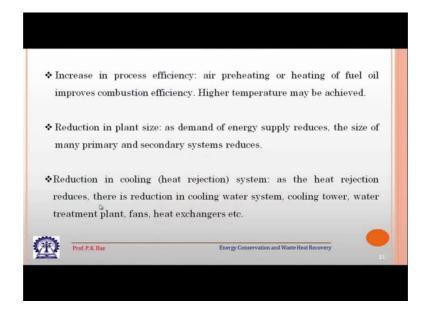
Then increase in process efficiency: increase in process efficiency waste heat whatever we are getting air preheating is a good option utilizing waste heat or one can even heat the fuel oil before it goes to the combustion chamber.
