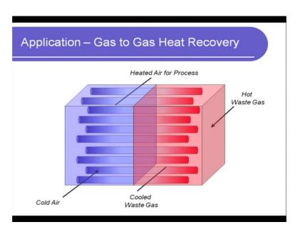
So, I will show you the slide over here once more if you recall this there were 2 chambers on one side we had hot waste gas which otherwise would have been wasted. So, that is the waste heat that we want to recover. On the other side we have a cold air it can be any other fluid also, but at this point let us say we want we have cold air supply and what we want heated air for some application or for some process.
