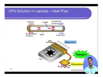
But; however, I cannot put the fan and heat exchanger right at the CPU location why because I do not have the space. So, therefore, I have extraction at one place rejection at another place I need to connect them with minimal temperature drop and the way to do that is using a heat pipe and the way I heat pipe works you have already seen that through that. So, through that animation all right.
