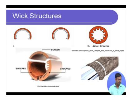
All right, so these are some of the applications of heat pipes for waste heat recovery and let us look at now on we were talking about the wick. So, what is a typical wick structure? So, the wick in the heat pipe can be of various types the 3 most important ones are shown here, the one is a wrapped screen. So, you can take a wire mesh or wire screen mesh and then take a few layers and wrap it on the inner surface of the heat pipe the
