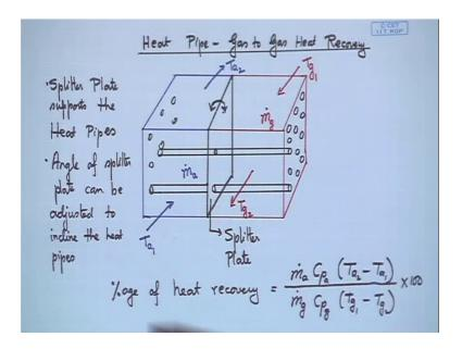
So, let us draw a schematic of this and so let us say heat pipe. So, I will use black ink Heat Pipe for Gas to Gas Heat Recovery, again keep in mind I am saying gas to gas it can be any fluid to any other fluid also . So, let us talk about these 2 chambers that we were drawing before on one side we have a hot chamber through which my hot gas is passing.
