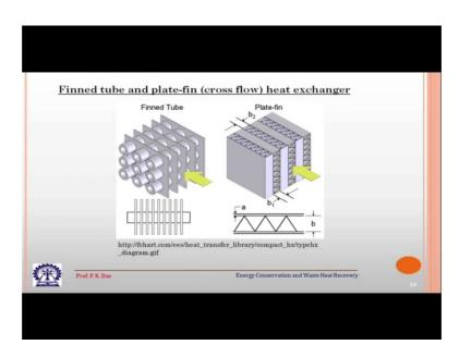
This is your fin tube heat exchanger or rather this is this there are two2 heat exchangers shown both uses extended surfaces or fins for augmenting heat transfer. Let me tell you that if we consider that there are 2 streams one is a liquid streams another is a gas stream.
