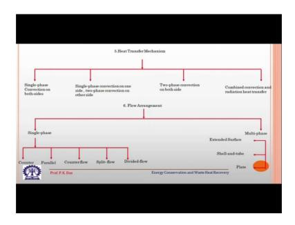
Next classification if we see the next classification is based on heat transfer mechanism, it could be single phase if there is no phase transfer both the fluid streams they are exchanging heat, but both of them are in the original phase itself there is no phase then it is single phase. Then single phase convection on one side, 2 phase convection on the other side, then 2 phase convection on both the side combined convection and radiation which can be there in kind of a in a boiler.
