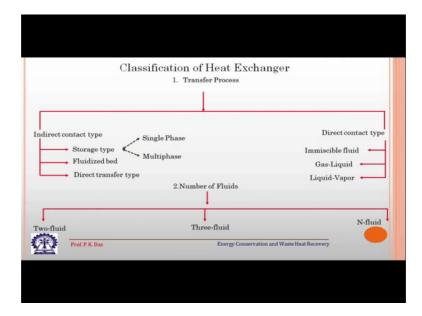
So, depending on transfer processes heat exchanger can be classified and most of the heat exchangers are in direct contact type; that means, 2 fluid they will not contact each other they will thermally contact or thermally interact with each other through some sort of a solid wall.
