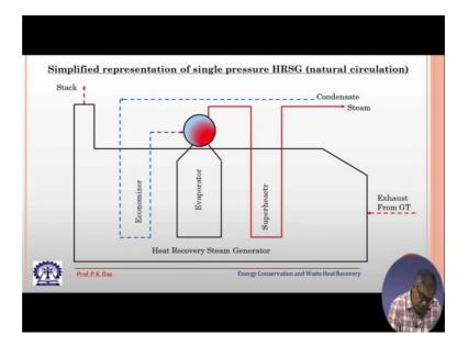
So, you see this shows schematically one single pressure HRSG the arrangement here is horizontal which is very common and Exhaust from the gas turbine which is high temperature gas.
