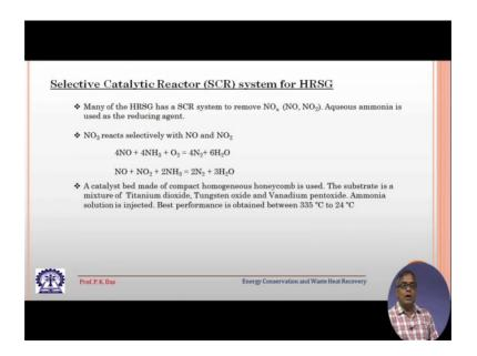
Now in many of the many of the HRSG will use a selective catalytic reactor or SCR. So, that will operate on NOx particularly it will operate on NO and N 2 aqueous ammonia is used to reduce as the reducing agent.
