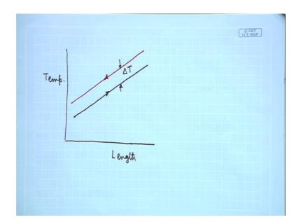
So, this side is your temperature and let us say this side is your length length of the HRSG and if it is ideally a counter current type of heat exchanger HRSG is counter current type of heat exchanger. So, the cold fluid steam could have gained it is temperature like this could have been ideal and for a good heat exchange, one could have kept this delta T uniform along the length as far as practicable.
