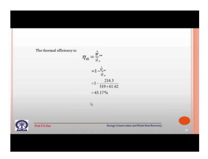
So, thermal efficiency will be W net W dot net divided, but divided by Q dot. So, here you see addition of both the turbine work that is given and here the addition of both the work sorry both the heat addition in the boiler and in the reheater. So, that is given and with that we get an efficiency of 43.17 percent. Now let us go back to the first cycle diagram I like to conclude this lecture, but before that I like to give you some messages which you can take back.
