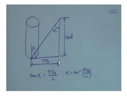
This is your cylinder this is your helix and you unfold it so that you get a triangle what's this triangle having is having this side equal to  $\pi^*D_P$  that means the circumference of the pitch circle okay circumference of the pitch circle it rides up by the lead in one rotation so this must be equal
