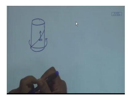
If we have a particular you know cylinder on that by some means if we are tracing a line okay this line will be executing a helix I mean the tracer will be executing a helical line if you have circular motion of this disk combined with straight line motion of this say pencil if they are you know proportionally moving that means if this is moving a certain number of units this moves by a proportional number of units and this particular proportionality is maintained.
