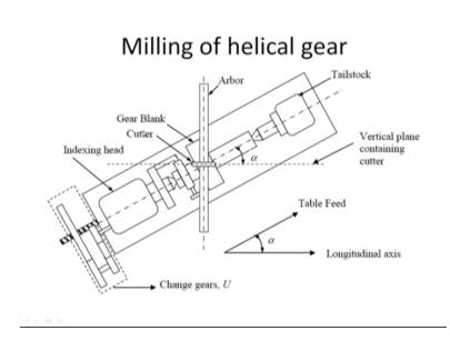
So to start with by the way we have finished most of the discussion on differential indexing so let us start with helical gear cutting on the milling machine what do we have here we are seeing the milling machine from the top the milling machine table you have already seen this one in the previous lecture and let me quickly identify the various parts which are present here.
