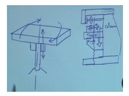
Table and there is one vertical screw provision for a vertical screw okay and this vertical screw is supported here and this one a there is a provision to have a nut here which makes the table move up and down, okay. So this whole thing then seen from the side looks like this table and screw and it can move on the milling machine up and down but what is the column that we are talking about this is the column okay.
