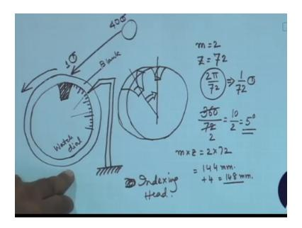
If you look at this particular gear okay if I have to remove this material in order to create teeth in that case after this has been cut I have to give it a rotation of this much and here I have to give a rotation up till this point, how do I give that? So let us do some calculations to find out how much is this rotation is supposed to me, so once again let us take some specifications say module equal to two numbers of teeth equal to say 72 okay.
