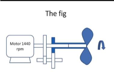
This one will be 90 teeth, 30 teeth, 40 teeth sorry 80 teeth, 40 teeth and therefore the fan will be rotating on the required speed, okay.
