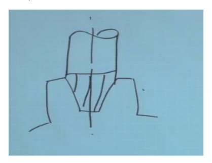
Have a look please this is the N milling cutter okay, it rotates this way and removes material it is not as popular as the other configuration of rotary disc type form milling cutter okay.
