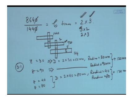
Their diameters are so z = 30 diameter equal to  $2 \times 30 = 60$  millimeters and radius = 30 millimeters and Z = 90 naturally we can pass all these we can say radius will be equal to naturally three times of this, how much is that? It will be 90 millimeters this one when added together will give us 120 millimeters Center distance so this is quite satisfactory we can use 30 teeth gear with 90 teeth and achieve 1:3, 3:1 speed increase.
