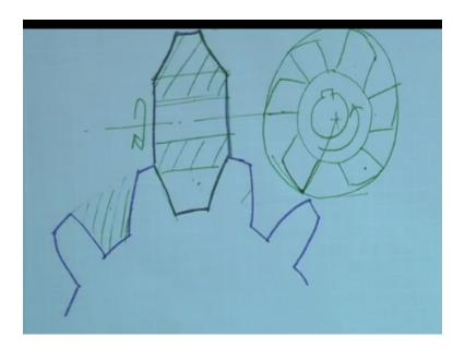
Now the cutter, how does the cutter look like? The cutter looks like I want to cut off this portion so the cutter exactly conforms to this particular shape rather let us use a different color this is the cutter so it looks like this in what way this is its axis of rotation okay it might not move right up to this portion because there will be teeth like this why have I given no section line here actually here also there will be no section line.
