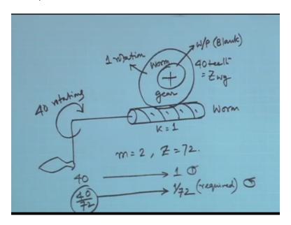
The indexing head basically consists of this is the main working part of it, this is a warm now you are quite conversant with the worm and the worm gear can be here up can be here to the side etc let us draw it up it has a worm gear connected to it worm gear what is worm gear doing, this one has say 40 teeth and this one is say K=1, so if I give 40 rotations here this is going to give me one rotation only.
