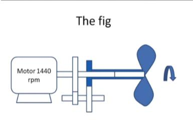
In which the motor is rotating here and there are two gears which are reducing a increasing the RPM in this ugly shaft these two gears are sharing the RPM and this is finally giving it to another gear which is loosely fitted on this shaft and connect it to the fan so that ultimately the fan rotates at the required rpm, what sort of increase is there so if you divide the initial rpm sorry if you divide the rpm.
