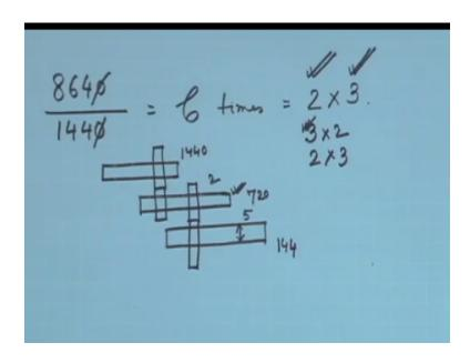
And let us work it out on the piece of paper 8640 rpm by 1440 rpm I think off and I if you calculate you will find  $6 \times 4$ , 24.  $6 \times 4$  times increase of rpm is required and as shown in the figure it has been the it has been provided that we should try to achieve it in two steps, now this is  $2 \times 3$  so let us have a multiplication of the RPM 2 times and then the multiplication in three times but should we first do three and then two or then two and then three.
