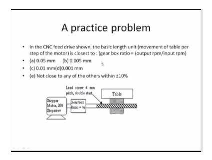
Another one slightly different configuration but this will also help you to understand the application of gearboxes later on. In the CNC feed drive shown the basic length unit that is the movement of the table per step of the motor so what do we have we have a CNC system in which there is a stepper motor which rotates in steps to cover one rotation in 200 steps.
