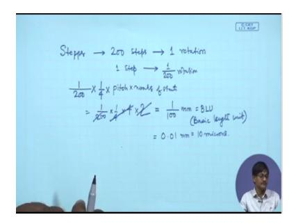
So we have stepper 200 steps one rotation, one step  $1/200^{th}$  of a rotation all right, therefore I start with  $1/200^{th}$  of a rotation multiply it by the gearbox ratio 1/4th multiply it with the lead screw lead, lead screw lead is pitch which is let me write down here pitch into number of starts equal to  $1/200 \times 1/4^{th}$  into which is 4 mm and it is double start so multiplied by 2 equal to 1/100, 1/100 millimeters.
