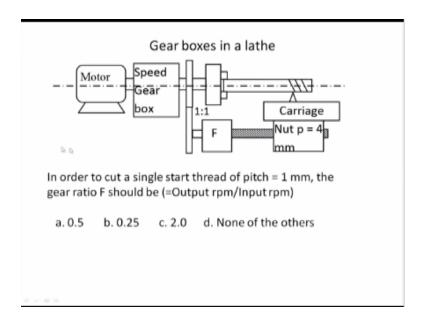
In order to cut a single start thread of pitch 1mm so by the time the spindle rotates once the carriage should be moving by one mm okay, the gear ratio F should be that is output rpm by input rpm equal to these, these, these extra, so let us have a look the nut is having four millimeters pitch, here there is 1:1 ratio so by the time the spindle rotates once this particular shaft will also rotate once.
