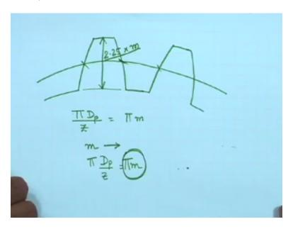
If this be how is module affecting its shape or size we find that if we draw the pitch circumference from here to here okay this distance is constant for all gears having same module so module defines this distance on all gears having the same module so this distance is equal to  $\Pi D_P/Z$  okay so module is relevant to the gear teeth by this dimension and if we assume that these two dimensions I mean this is equal to this then this one is also perfectly defined by module.
