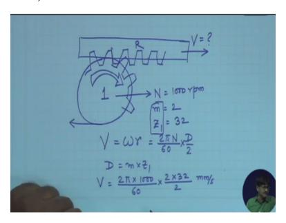
Now let us take the case of rack and pinion let us take a simple problem also say I have this as a gear depiction of a gear and this as the rack. Suppose I give this information this one is rotating and is called 1 and this is called R, for R I am interested to find out the velocity it will develop, and here I am having N = 1000 rpm module equal to 2, number of teeth equal to 32 what will be the speed developed by the rack.
