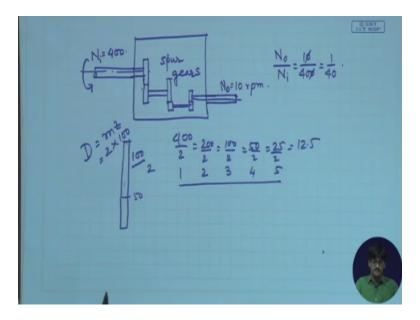
If I am having say an input shaft with rotational speed equal to 400 and if I tell you that make a gearbox into which it is moving in put whatever ordinary gears that we have discussed up till now spur gears I will come to this term spur gears, but whatever spur gears that you can put in
