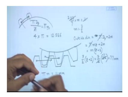
It is in mesh with opinion having 20 teeth outer diameter of the pinion is so this is the pinion etcetera, so we need to find out what is the outer diameter of the pinion now as they are meshing therefore linear pitch of the rack must be equal to the circular pitch of the gear circular pitch once again is  $\pi xm$  okay, so  $\pi xm$  must be equal to 11 millimeters, let us use this part this is clear so we have 22/7xm=11 this and this they will cancel and m=7/2 okay.
