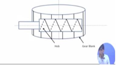
Now coming to this how do we decide this problem also we have identified, how do we decide whether a particular hub is correctly aligned with the work piece or gear blank, for that let us see we are taking the case of our spur gear with straight teeth and this is a right-handed helix so the dotted one is the one which is touching or on the side of the gear teeth in contact with a gear teeth.
