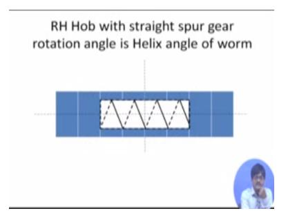
Second case let us try it out the blue one is the gear to be cut and these white vertical lines they are the traces of the teeth. Now let us give it a rotation and see what happens yes, this seems to be it therefore the dotted lines are matching with the direction of the teeth being cut and therefore we say that for cutting a spur gear with right hand hub the rotation angle is simply the helix angle of the worm okay.
