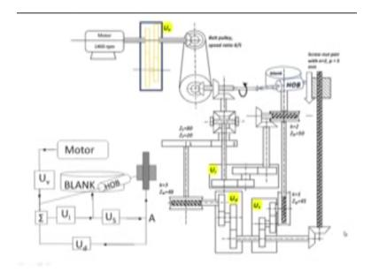
And therefore we move on to now the feed gear box we will determine how feed gear box is decided let us see where feed gear box is situated the feed gear box is situated here and the feed gear box we can notice is here, how is the feed gear box you know influencing the operation of the machine we say that is the hob is moving down too fast in that case it creates a problem that the surface which is left it is going to be too rough let me draw a figure and show you.
