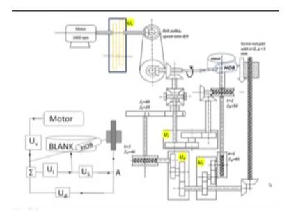
So for that one thing in the figure where are the lead change gears the lead change gears are US coming here if you if you follow me from the point it is a bifurcation on one side we are serving the screw on the other side we are serving the lead change gears normally when you are cutting spur gears they do not take part in the cutting action but now they are going to rotate and they are going to get added up to the rpm which is imparted by virtue of hob rotation from the other input side.
