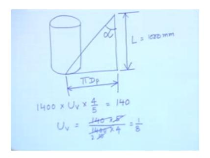
1400 x UV x belt pulley 4 that's it, after that there is no other member affecting the RPM so this must be equal to 140 rpm as given in the problem. Let us find out what UV comes out to be UV comes out to be  $140/1400 \times 5/4$  equal to this, this we have a 10 here this, this we have a 2 here so it is 1/8. UV = 1/8 okay.
