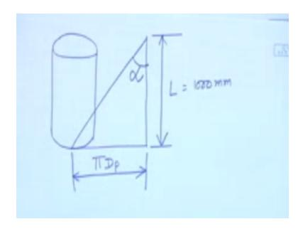
If you unroll one tooth this is the lead equal to thousand millimeters this is the circumference equal to  $\Pi D_P$  mind you here it will be equal to M normal module into Z number of teeth divided by Cos  $\alpha$  where  $\alpha$  is the helix angle, helix angle okay.
