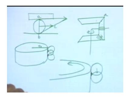
If this is the blank and this be the you know idealized position of the hob there is only a point-to-point contact so after every rotation say this particular meridional position this radial position we call as RX so it is going to come back to RX after every rotation one rotation it is here second rotation is here third rotation is here so it leaves behind these small scallops of material how does it look like in a blown-up figure it looks like this.
