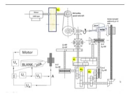
Let us go back here and let us see how this is implemented first of all how is the hob coming down well just as it is rotating it is also attached to this nut this nut is attached to the hob so that if the nut goes down the hob goes down as well so who is making the nut move down this particular screw vertical screw which can be seen here this is rotating and it is bringing the nut you know further and further down.
