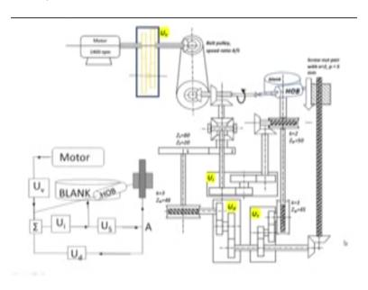
So with this in mind let us look at the schematic figure now so we will say that I will achieve a thousand millimeters that is lead amount of motion in this particular knob for that I will have a certain number of rotations of this screw with these many rotations I enter UD that means the lead change gears and from the lead change gears I go to the differential I calculate whatever ratio differential offers me when the other output is off and this input is on and I pass through UI once again.
