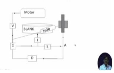
The set-up for helical gear cutting
