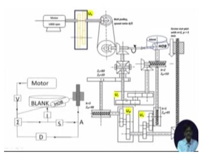
How to work with the differential in the differential items suggest that when you are finding all the initial values consider the output rpm of the lead change gears to be 0 and that way you can first set the values of V I and S that means Uv  $U_I$  and  $U_S$  can first be found out by considering the output of the lead change gears to be 0 rpm and then we will find out the final value of D so with this we come to the end of the 16<sup>th</sup> lecture thank you very much.
