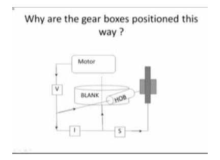
And if you look at this was the accepted position and this was the changed position and we noticed that the location of I in this particular position unfortunately is going to change the HOB rpm and that would result in a different cutting speed and that is going against our basic resolution that one gearbox should affect only what it is intended to and nothing else change in speed should be controlled by the change in UV change in speed.
