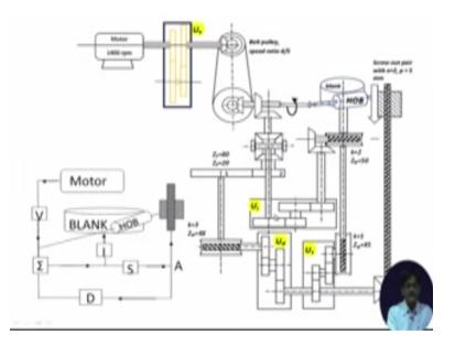
Let us have a quick look here for example is there any mechanism which is not known to us how it operates we have bevel gear etc... the differential the differential is something which is at present not known to us I would suggest that when you are solving for the initial part of the problem consider that you are not cutting a helical gear at a by the way have I provided the helix angle.
