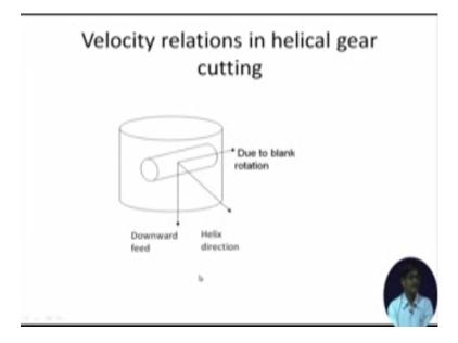
This is the velocity relation which we have already discussed that means the hob has downward motion and the blank will be given extra rotation because of which there will be a tangential motion the resultant of both the velocities will give rise to the helix direction. (Refer Slide Time: 16:03)
