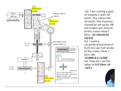
We have up till now finished up to this point that is the second question and we were discussing just to pick up the threads we were discussing the cutting of the spur gear on the fellows gear shaper the fellows gear shaper works on the principle of generation okay, so last question that we have left is how do I set the value of U I, now if you if you recall the discussion in the last lecture UI is situated here and UI is decided by the number of teeth that we are going to cut.
