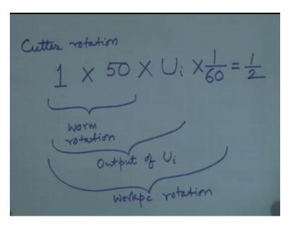
First of all cutter rotation, cutter rotation 1 we put the cutter rotation to be 1 and then we multiply it by so it is the same as the worm rotation and then we multiplied by 50/10kay, the reverse ratio to get the worm rotation, fine after that through the bevel gear pair we come to the main line it is just like a car backing off from a buy lane onto the main road, so you are going reverse and after reversing you come to the main road.
