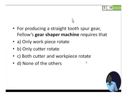
For producing a straight tooth spur gear the fellow's gear shaper requires that only work piece rotate only cutter rotate both cutter and work piece rotate none of the others so which one is correct only the work piece loaded but the basic condition which has to be satisfied in case of gear shaping is that both the work piece and the cutter should rotate as if they are rolling against each other as finished gears.
