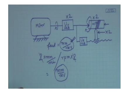
And I think that will make subsequent discussions extremely clear on the lead we have a motor from which we are drawing power and if you remember we have the location of speed gear box let us call it SGP speed gear box here and after this just like as in the gear shaper we have the spindle to contain the work piece and we draw the power from here for US feed gear box and from here you might be having a lead screw and you can mount your nut and the cutter this way.
