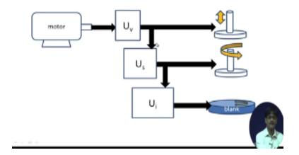
So let us have a look at this particular interconnection what do we notice here the motor is first of all serving UV the speed gearbox, so rotation of the motor everything we have you know represented symbolically, so it means that the power is flowing from the motor to the speed gearbox how does the power flow, so the motor shaft is rotating and that shaft goes inside the gearbox UV there \will be a cluster of gears and these cluster of gears would be changing the RPM.
