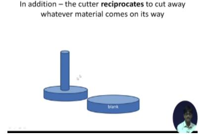
This is the cutter this is the blank and the cutter is also moving this way together with rotation of the cutter rotation of the blank as we have seen before and movement of the blank towards the
