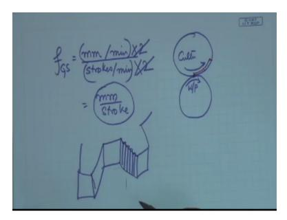
Millimeters so the feed in case of gear shaper in case of gear shaper millimeters per minute by strokes per minute strokes per minute is getting doubled millimeters per minute circumferential movement okay it is like this is the cutter this is the work piece and therefore this one is rotating against each other and therefore the movement it suffers say I will draw with a different color the movement it suffers per stroke this becomes double this becomes double per minute sorry per
