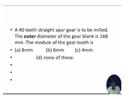
40 teeth straight spur gear is to be milled the outer diameter is 160 millimeters the module of the gear too this, so how do we solve this question we say that the outer diameter of the gear blank in case of straight spur gear is.
