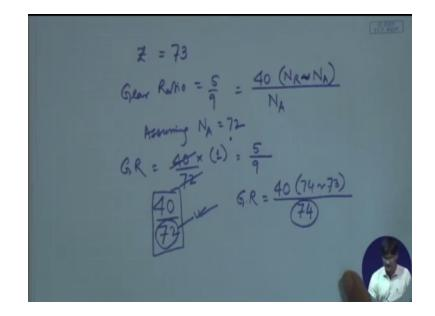
If you look at this piece of paper so we write here read is = 73 teeth okay gear ratio = 5 / 9 that must be = 40 / N available x n required - N available let it has a difference because we are not considering the sign of this moment, so if this is 5 / 9 we can we can have right if we take assuming let us try the solution assuming N a to be 72 okay then gear ratio comes out to be 40 / 72 x1 = this cancels out how many times can cancel / 85 are 40 + 9 x 8 72 that is it.
