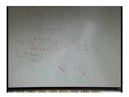
So, when you have pipes in parallel, let us try to make a sketch of a may be a situation like this. So, you have 2 pipes which has sort of connected in parallel; that means, they are branching of from just let me sketch it in a bit of a different way.
