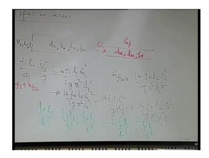
So, pipes in series it means that you have let us say that you have 2 pipes like this, the name series is obvious they are connected one after the other. So, you have let us say that the diameter of the first pipe d 1, the average velocity V 1, length l 1 friction factor f 1 and for the pipe 2 corresponding things are there.
