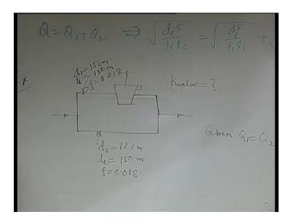
So, you have 2 pipes, 2 pipe lines and these 2 pipes the upper one is d 1 is equal to 15 centimeter, and length is 150 meter, the friction factor is a constant which is 0.018. The other pipe is the diameter d 2 is 12 centimeter, the length 1 2 is 150 meter and the friction factor is the same 0.018, it is given that Q 1 is equal to Q 2.
