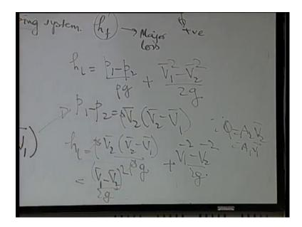
So, the head loss we can calculate. So, divide by g into call it a unit of a head; head loss is P 1 minus P 2 by rho g plus z 1 square minus V 2 square by 2 g.
