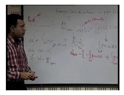
So, let us look into a bit more details of the energy considerations in the pipe flow. The objective will be to figure out that how the head losses are related to the total energy balance.
