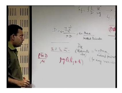
So, the one of the important things that the diameter is the function of the cross sectional area and the perimeter, so what is the cross sectional area, pi d square by 4. And the perimeter is pi d. So, you can see that we have to adjust it with a 4 to get back the diameter.
