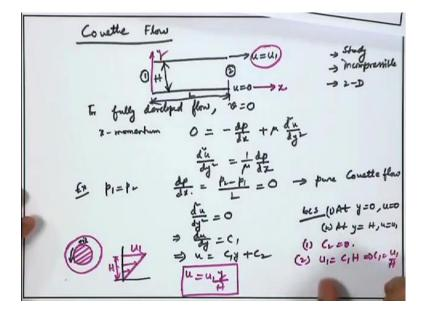
Let us say that the bottom plate is stationary and the top plate is moving toward the right with a velocity u 1. The gap between the plates is small and the flow is fully developed. Now you may ask the question that why are we studying this. Have you ever seen somebody pulling plate on the top of another plate? I mean I have never seen this kind of a situation.
