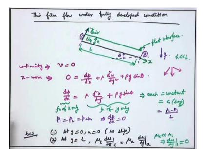
Let us say, that there is an inclined plate and the plate is incline at an angle theta with the horizontal, whereas, the gravity is acting vertically downward fashion. We set up the x and y axis such that x axis is along the inclined plane, and y axis is perpendicular to that. And there is a thin liquid film with a flat interface. If it is a curved interface it is a significantly more complicated problem that we will not take up in this particular lecture.
