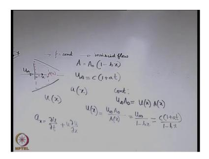
So, we have a nozzle like this and it is carrying a fluid with density equal to constant and some other input data are given for the problem the area of the cross section of the nozzle; it varies with the area of the cross section of the inlet in the following manner where x is the coordinate measure from the entrance.
