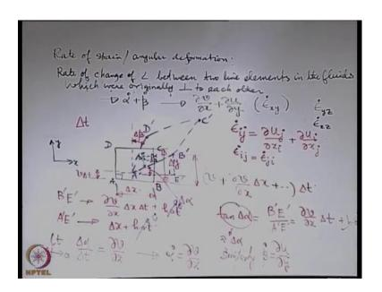
So, angular deformation of fluid elements; let us say that we start with rectangular fluid element like this when we are thinking about angular deformation the deformation is in terms of change of an angle and that angle change may take place in a prime. So, although the general fluid element is 3 dimensional element, but you can always take a 2 dimensional element and consider the deformation in the prime because no matter how
