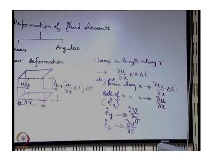
Next what we will do we will start analyzing the deformation of fluid elements. Why this is very important because we have seen that fluids are characterized by deformation they undergo continuous deformation on the under the action of even a very small shear force and the relationship between the sheer force and or the shear stress and the rate of deformation is something which is unique to the constitutive behavior of different fluids.
