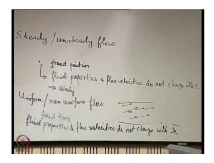
First concept is steady and unsteady flow. When do we say that a flow is steady? Whenever we are trying to focus our attention at a point say by following the Eulerian approach, we are interested to see that the flow velocity of fluid properties at that particular point are changing with time or not.
