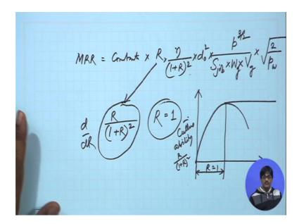
And what is MRR equal to? If you have a look here, MRR is equal to all sorts of constants multiplied by R into eta 1 plus R whole square into you know d 0 square divided by s job multiplied by width of groove, multiplied by velocity of groove, p to the power 3 by 2, 2 by. So, all these things I am sure you will be remembering better than
