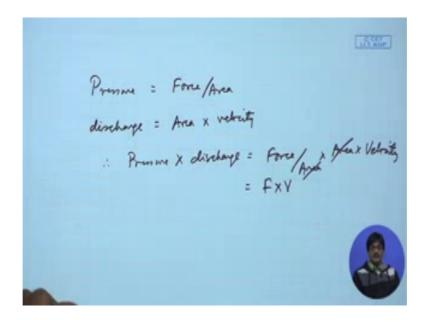
Pressure equal to force by area and discharge equal to area of cross section area into velocity. Therefore, pressure into discharge becomes equal to force divided by area into area into velocity and therefore obviously, it is equal to force into velocity, which we know to be power force into displacement is energy and force into velocity is power.
