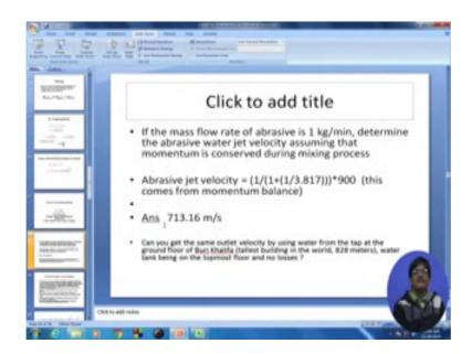
So, this way we can find out the final abrasive water jet velocity from the initial velocity. So, with this let us draw an end to the 17th lecture. In the 18th lecture we will take harder problems, harder numerical problems so that we become conversion with the working of the machine and it is process capability.
