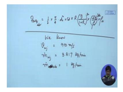
This is what we start with, we know that velocity of water jet is equal to 900 meters per second. And water jet mass flow rate, mass flow rate of water jet was equal to 3.817, 3.817 kgs per minute ok.
