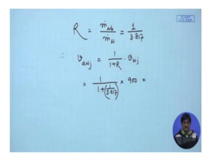
It is equal to mass flow rate of abrasive, by mass flow rate of water and that is equal to 1 divided by 3.817 and therefore, velocity of the abrasive phase sorry, velocity of the abrasive water jet must be equal to 1 by 1 plus R into velocity of water jet. So, this is equal to 1 by 1 plus that is it yeah.
