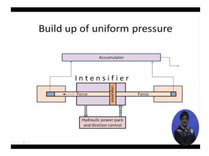
Let us now have a look at the base I mean schematic of the supply of high pressure water. So, first of all hydraulic power pack with a direction control valve it is responsible for putting in you know pressure at the I mean high pressure water; that means, which is coming out of the hydraulic power pack, say at 100 bars it is coming here.
