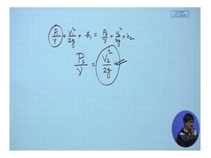
Let us say we have P by gamma plus v square by 2 g plus h velocity head pressure head and this is the height. So, this one will be equal to if we take another position P 2 by gamma v 2 square by 2 g plus h 2. We start from a place where there is absolutely no velocity, no height same height as the previous one. So, in that case it is called stagnation the water is starting from stagnation and only the pressure head will be existing.
