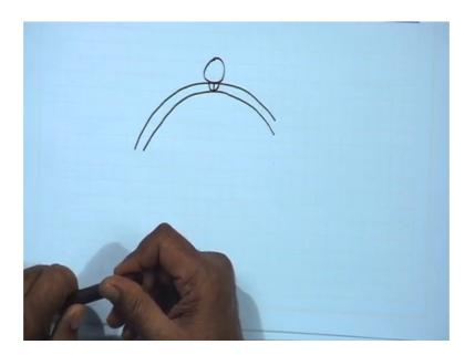
If this is the helmet body and if this is the ball, the ball should create you know hemispherical chunk whose radius will be equal to the thickness of the helmet. In that case we will consider the perforations to have been performed successfully. Radius of the indentation should be equal to the thickness of the helmet. So, what is given after that? The minimum height he or she should program the drone to reach in order to perforate the helmet of a target at sea level is nearest to, ok.
