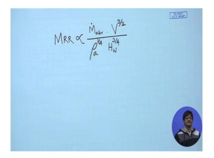
Once again we remember M RR is proportional to M dot abrasive into V to the power 3 by 2 divided by rho to the power one-fourth and H to the power 3 by 4. This one is work piece, this one is abrasive, this one is abrasive. So, in this case if V is being changed; V is being changed; obviously M dot is not change because nothing like that has been stated.
