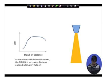
Standoff distance, what the standoff distance mean? Standoff distance means that whenever we are having the end of the tool as a nozzle. And from the nozzle abrasives are coming out at high speed, then the distance between the tool sorry the nozzle tip and the work piece surface that is called the stand of distance. And this is generally of a very low dimensional value say, 0.5 millimetres by common. So, a very small distance is there.
