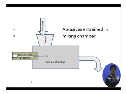
This is the figure of the mixing chamber, gas is coming in at high pressure and inside the mixing chamber abrasives are coming through the hopper and they are getting entrained here. At the end of the hopper there might be are you know a sieve a sieve through which the abrasives can pass and this whole thing might be mounted on a vibrating chamber so that the abrasive feeding becomes easier.
