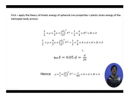
Let us have a look at the calculations. First apply with a theory of kinetic energy of spherical iron projectiles equal to plastic energy strain energy of the helicopter body armour. Remember the helicopter is covered by TIB two plates which have some 3200 kg of per millimeter square or something like that. So, we will come back to those values later on. First of all let us see what has been tried out here.
