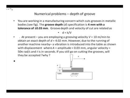
So, this problem deals with you are working in a manufacturing concern which cuts grooves in metallic bodies. So, there is a metallic body and you are cutting a groove. It is a brittle metalled material.
