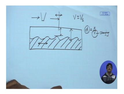
Now, what is going to happen here is that if you now look at this particular piece of paper, so if this is you know say top surface of the metal piece and I am having a grooving velocity of this type, but if there is a vibration setting on the table while the grooving element or the nozzle that is still at the constant velocity. Therefore, this velocity will have a reciprocating velocity impressed upon it. So, it will be V plus minus V1 coming from the vibration.
