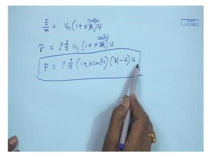
G is per unit mass, MG, sorry, but unit weight, okay. So therefore energy added or the head added per unit mass will be, therefore head added per unit mass will be E by M will be simply V R1 + K VR1, VR1 one + K VR1 into U, U is the blade velocity. Okay. Now if we want to find out the total power that is being delivered to the rotor by the fluid then we have to multiply this head given by the fluid to the rotor into the mass flow rate. And what is mass flow rate?
