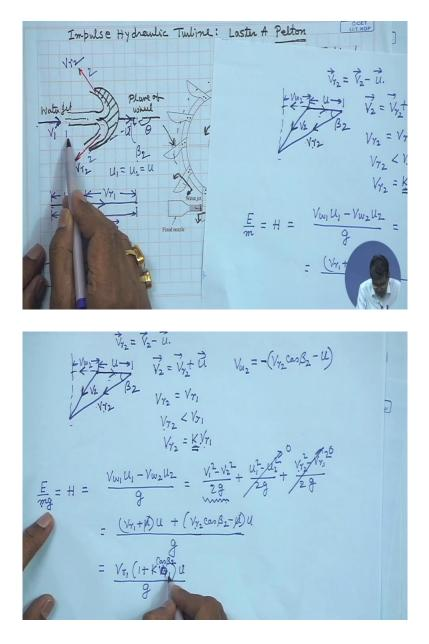
Now we draw the velocity vector or the velocity triangle for the outlet. For the outlet we will draw the velocity vector or the velocity triangle at the outlet. Okay. Now the velocity vector at the outlet if we draw, we see this picture, it will be enough. Now here, this is the VR2, so therefore here  $1^{st}$  we draw, now we write one thing that VR2, how to draw the velocity vector or the velocity triangle, VR2 is V 2 - U2. VR2 is V2 - U2, U2 is U, that is U only.
