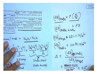
So that U1, U2 I find out U1 this way, U2 this way, we can find out and then what we do, we can find out the work done. Now if we know this work done for an incompressible situation, we can write that Delta P stage is nothing but rho times, this work done per unit mass, work done per unit mass. That means you just multiply with rho, this with rho, you get the Delta P per stage. Total in the stage you find out the Delta P. Okay, fine. Now static pressure rise is this one.
