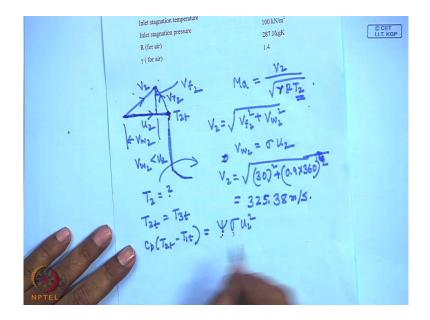
Now let us solve problems. So we have discussed the principal of, the characteristic curves, the concept of surge, the surge line, the maximum efficiency line and the choking line. Now let us consider this problem. A centrifugal compressor has an impeller tip speed 360 metre per second, this is the impeller tip speed. Determine absolute Mach number of flow leaving the radial vanes of the impeller and the mass flow rate. The following data are given, so data are given.
