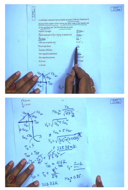
Again I will show you the problem that impeller speed 360 metre per second, radial component of flow velocity 30 metres, slip factor is 0.9, flow area at impeller exit 0.1 square, it is not now required. Power input factor is given, isentropic efficiency given, inlet stagnation temperature, inlet stagnation pressure, then R and gamma. So here what is required, power input factor which is given as 1, the slip factor which is given is 0.9, U2 is 360 metre per second and T1 T is 300 K, we get T2 T.
