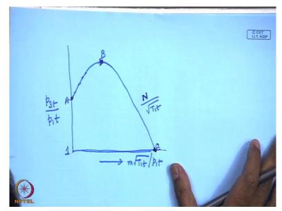
P3 T, that is the pressure ratio P1 T versus the nondimensional mass flow, normalised, sorry normalised mass flow P1 T, the curve looks like this, I tell you, this curve looks like this. The curve looks like this, I will explain, let me 1<sup>st</sup> draw the, label the curve. Now I will explain, the 3 points are important points in understanding this. Now what happens, if you make an experiment and draw the points, you will get a curve like that.
