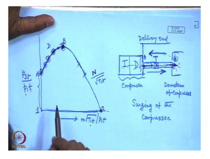
Now this part of the characteristic curve is having a positive slope and usually this part is unstable and is very difficult to have this part of the curve in practice. Rather this part, which is associated with the negative slope, that pressure rise and mass flow rate is stable, how I will explain you. Now let us consider a compressor like this. Let us consider a compressor like this, this is impeller, this is diffuser, this is totally the compressor. Try to understand this compressor.
