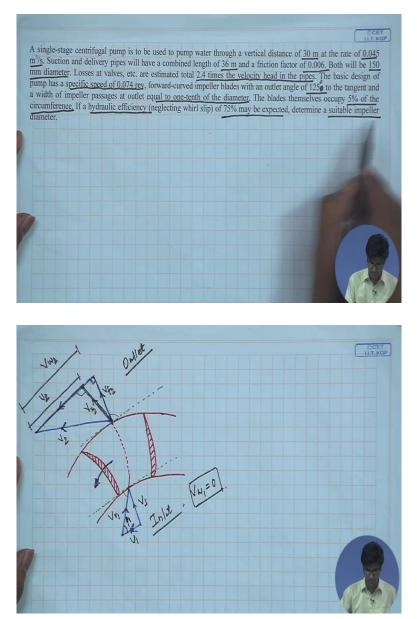
Today I will be solving some problems on centrifugal pumps. So let me start with the 1<sup>st</sup> problem. Let me read it out. A single state centrifugal pump is to be used to pump water through it what equal distance of 30 metre at the rate of 0.045 metre cube per second. Suction and delivery pipes will have a combined length of 36 metres, and a friction factor of 0.006,
