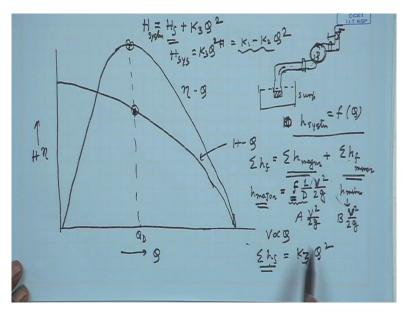
Now after that I will tell you about the pump and the system characteristics. Now let us consider the HQ characteristics which for a backward facing curve like this. Let us put H and it is Q and we have this HQ characteristics. Let us have the efficiency characteristic, the efficiency characteristic is like this. Now this H becomes 0 at some Q, that is also theoretically is seen that at some point, for example H is K1 - K2Q square. So at some point
