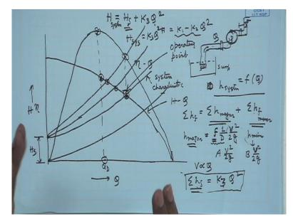
H system is equal to K 3 Q square. That means system will demand this type of head so that this pump can be in operation to maintain the flow, it contains all the losses and these minor losses also include the exit losses. That means the loss that is being incurred by the exit velocity. Okay. So therefore if we consider this thing as the system resistance with static lift HS, this can be expressed or this can be shown like this, here this is HS, let this HS.
