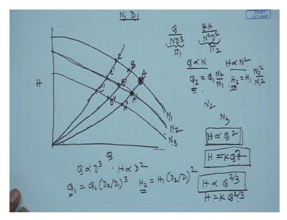
But I have shown it because this is in practical use. So therefore we, we are able to recognise the operating point of the pump in practical application. Now we will see the effect of rotational speed and the rotor diameter on the head discharge characteristics of a centrifugal pump. Now what is this? This is like this, that if we have a head discharge characteristics like this as already we have discussed, let us consider a head discharge characteristics like this.
