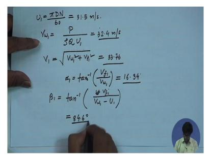
That is U1 is equal to pie DN by 60 where D is the diameter of the runner blade which is given, N is the rotational speed of the runner which is also given, the diameter of the runner is given as 1.4 metres and the rotational speed of the runner is given as 430 rpm. Substituting the values we get the value of peripheral velocity of the runner blade as 31.5 metre per second. So from the relation, from this relationship right now we know the value of U1.
