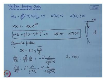
The next example that we are going to look at is that of a Uniform hanging chain. We have derived the equation of motion of uniform hanging chain previously and it looks like. So this is the equation of motion, this is the boundary condition at the fixed end. Now, once again we are going to attempt a solution with this structure and we obtain with the boundary conditions. Now in the case of a string of a uniform taut string.
