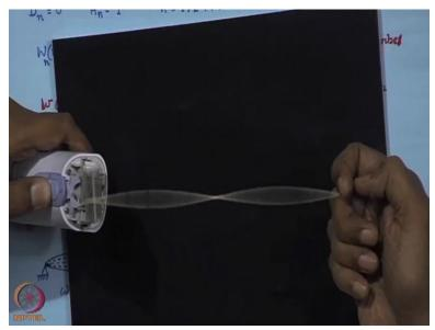
So this is the second mode of vibration of the string and I may also try the third mode which may not be visible very clearly, because the amplitudes are so small. But the second mode is quite clear and the first mode as well. So, this is what we have observed we have seen the first two modes quite clearly, third mode because the amplitudes are so small has been less visible and so on for the higher modes. But then, whenever, I pluck a string I actually excite a number of these modes.
