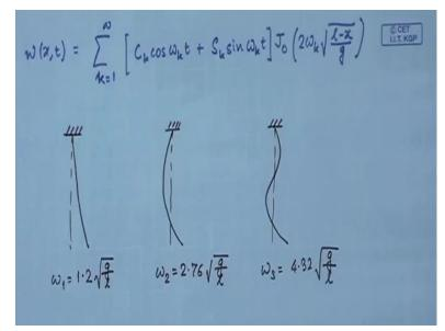
Now finally once you have this, you can write the general solution once again, using superposition. So these are the, these represent the modes, these are the Eigen functions and the modes of vibration of a uniform hanging string are defined by these Eigen functions. So the modes of vibration of a hanging string are defined by these Eigen functions and they look. So this is the first mode, this is the second mode and this represents the third mode.
