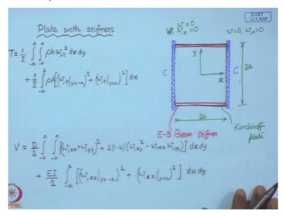
So we have a plate; we would like to see what happens when a plate is having stiffeners, a stiffened plate, the vibrations of a stiffened plate. We consider again a square plate. We consider that this plate is clamped on these two opposite edges. So, these two edges are clamped. The coordinate system is located at the geometric center. These sides are 2a and this is stiffened on these edges are free, but they are stiffened by beams.
