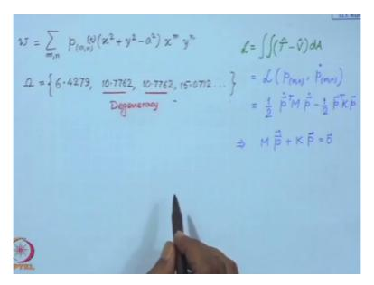
So, the expansion that we are using; so t these are the coordinates and that multiplied by the admissible functions; this is an expansion which we will substitute in the – in the Hamilton's principle. We will calculate the Lagrangian, so that is obtained as an integral over the area which now is actually dx dy. So, we will integrate over x and y to obtain the Lagrangian. Now, since we know all these functions and these are polynomials.
