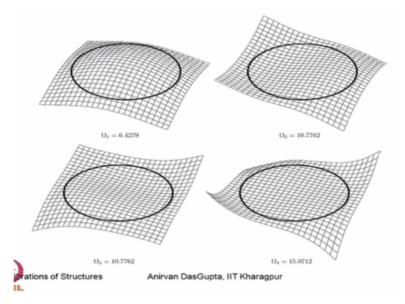
Now this figure shows the modes of vibration of the plate. So, this is the optimal radius which happens to be around 0.8, non-dimensional values. So the radius is 0.8. This is the fundamental mode; these two are the degenerate mode. As you can see that, this is nothing but a rotation of pi by 2, which is the symmetry of this problem because this is the square plate; rotation of pi by 2 is not going to change the problem.
