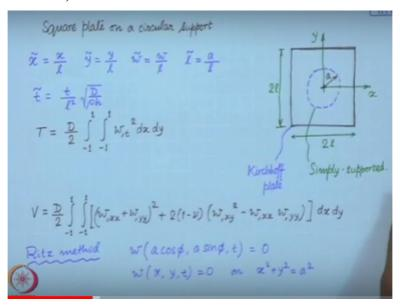
So, suppose this is a square plate of uniform thickness, which is supported on a circular support; it is simply supported. We consider that the length is 2l and this is at the geometric centre. Now, so we are looking at square plate on a circular support. This radius of this support circle is a and the side is 2l. now, we already have the kinetic and potential energy expressions; but I will make some simplifications, some non-dimensionalization.
