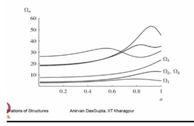
So, this figure shows, the variation of the first few non-dimensional circular Eigen frequencies with a. So this is the fundamental frequency of the plate with variation of a. So,
