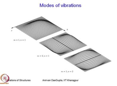
Now this figure shows the first three modes of vibration of this plate. So in the first mode there are no nodal lines where as the second and third they have these nodal lines. Now here you can see these two are the clamped edges, so the slopes are zero where as these are simply supported edges.
