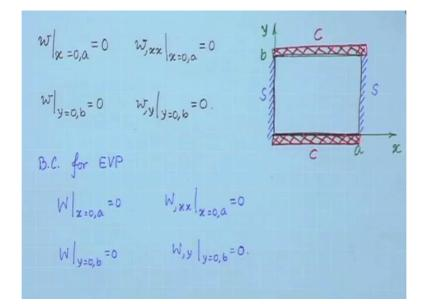
So in the x direction the length is a and here it is b again. Now we will assume that this side simply supported and these two sides are clamped, so these two are clamped, and these two edges are simply supported. So the boundary conditions for such a plate with such a boundary condition. So the mathematical representations are the displacement at x equal to zero and x equal to a they must be zero.
